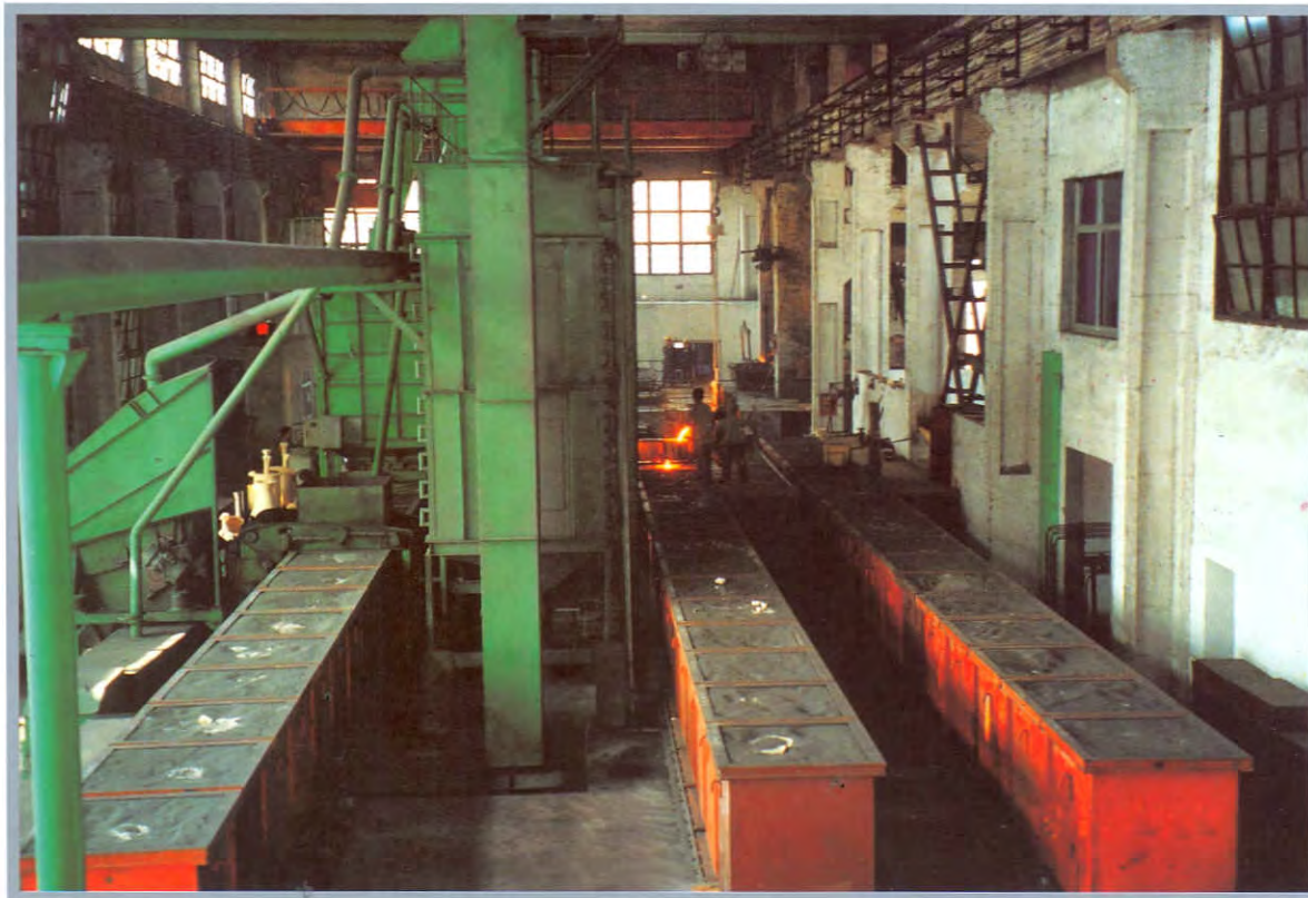
真空消失模管件生产线 Fittings production line by V-EPC process
