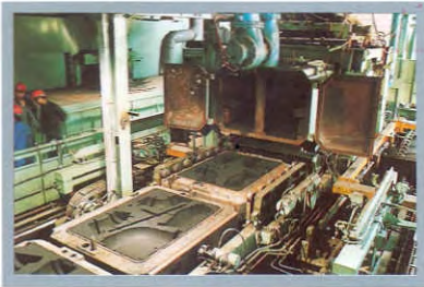
KW 高压造型管件生产线 Fittings production line by KW high- pressure molding process
