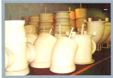
KW 高压造型管件生产线 Fittings production line by KW high- pressure molding process
