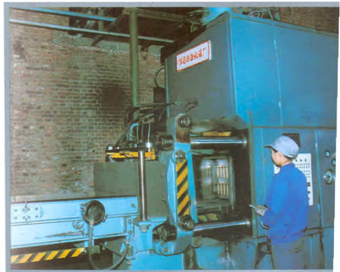
无箱挤压管件生产线 Fittings production line by flaskless squeezing method
